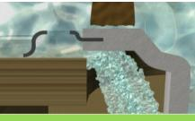
**does not seal to the floor** - only to the toilet with a wax ring
